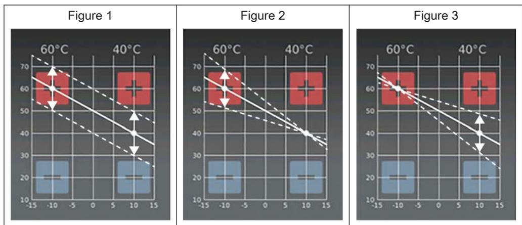
Depending on the situation, the heating curve can be adapted by tapping “+” or “-” at  $\pm 10^{\circ}\text{C}$  outside air temperature.
