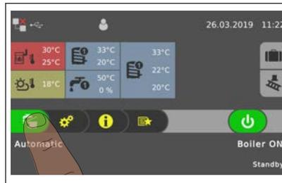
Depending on the type of boiler, there are several modes available which can be changed directly in the basic display of the touch display.
