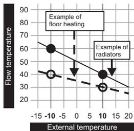
A flow temperature is calculated using the heating curve of the heating circuit depending on the outside air temperature and the two adjustable parameters “flow temperature at -10°C outside air temperature” and “flow temperature at +10 °C outside air temperature”.
