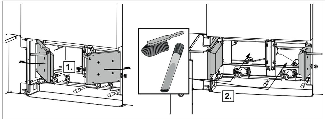
**NOTICE!** Only clean the grate and combustion chamber when the boiler has cooled down!
