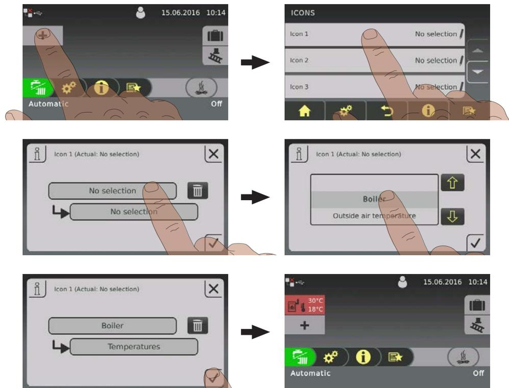
When using more than two store sensors, it is possible to have an information display with storage tank temperatures in accordance with the number of sensors. An information display that spans two areas is used.
