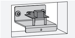
**NOTICE!** Fit the flow sensor as shown to prevent malfunctions!
