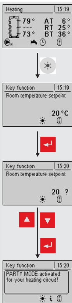
After the Party Mode key is pressed, an entry field to optionally change the “Room temperature setpoint” appears on the display. If no other key is pressed, daytime mode starts until the end of the next heating phase or until the automatic mode is activated for the allocated heating circuit with the preset room temperature.
