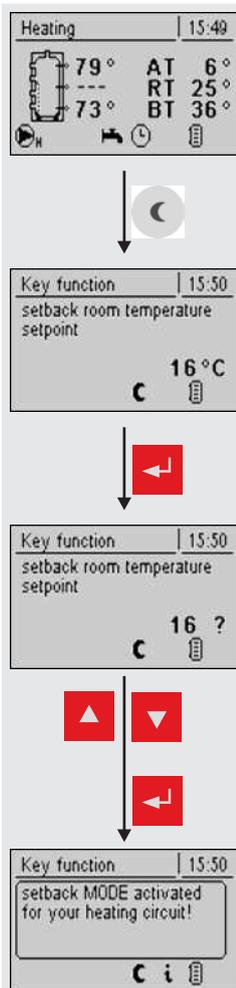
After the Setback Mode key is pressed, an entry field to optionally change the “Setback room temperature setpoint” appears on the display. If no other key is pressed, setback mode starts until the end of the next heating phase or until the automatic mode is activated for the allocated heating circuit with the preset “setback room temperature setpoint”.
