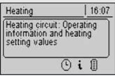
In normal operation (without pending fault messages) the info key can be pressed to display information or an explanation for every menu item or parameter.
