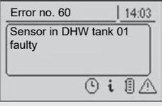
If a fault has been acknowledged after arising, but not resolved, this is shown by a warning symbol at the bottom right on the status line.
