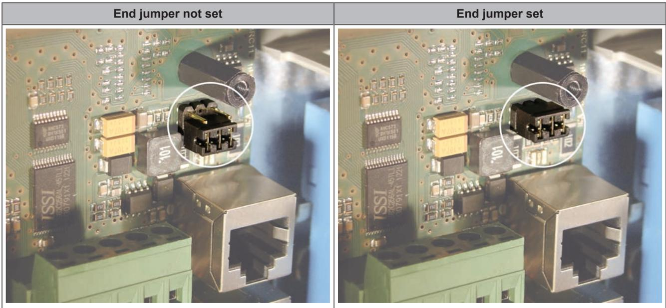
If the contacts at the base of the end jumper are not bridged (image left), it is referred to as “not set”. In this case there is no bus termination. If the contacts are closed (image right), the end jumper is set and the bus connection is terminated.
