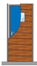
The pellet store door must be a fire door with a Class T30 fire resistance rating; it must have a seal. On the inside of the room you should install wooden boards to stop the pellets pressing against the door. Practice has shown that it is advisable to install an additional inspection window.
